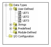
UDT1 contains a UDT2 and an array of UDT3
